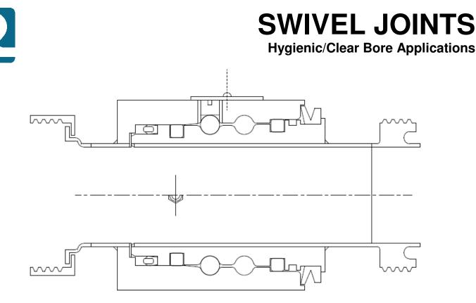
Rotaflow manufacture a range of swivel joints for customers facing the problems of fluid transfer where a clear bore is essential to avoid the problems associated with restriction of flow.
