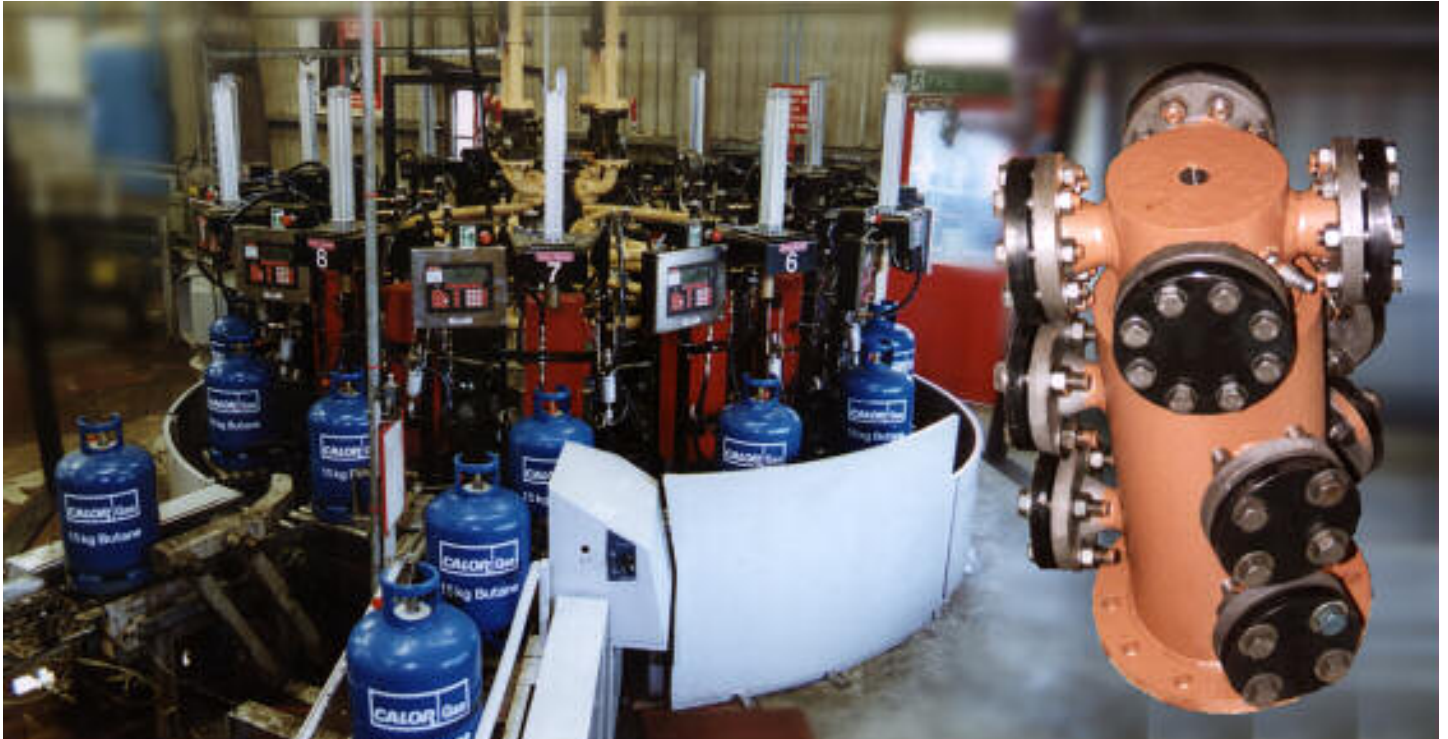
At the centre of the Calor Gas carousel is a Rotaflow swivel joint allowing either butane or propane to fill each cylinder in turn.
