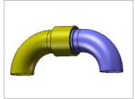
3. (40) Single swivel with two elbow stops to permit swinging lines in parallel
